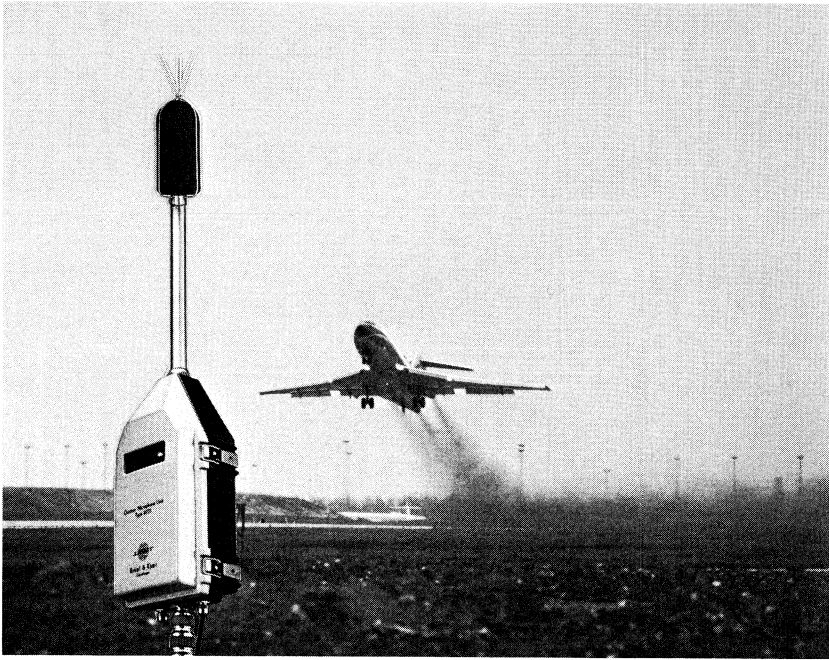
Fig.15. Outdoor monitoring of aircraft noise
